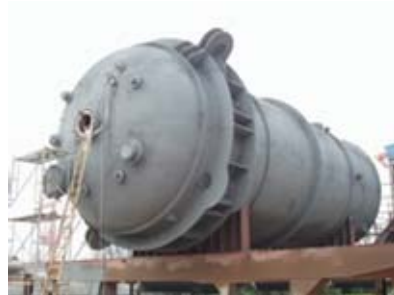
Oxidiser for a refinery
